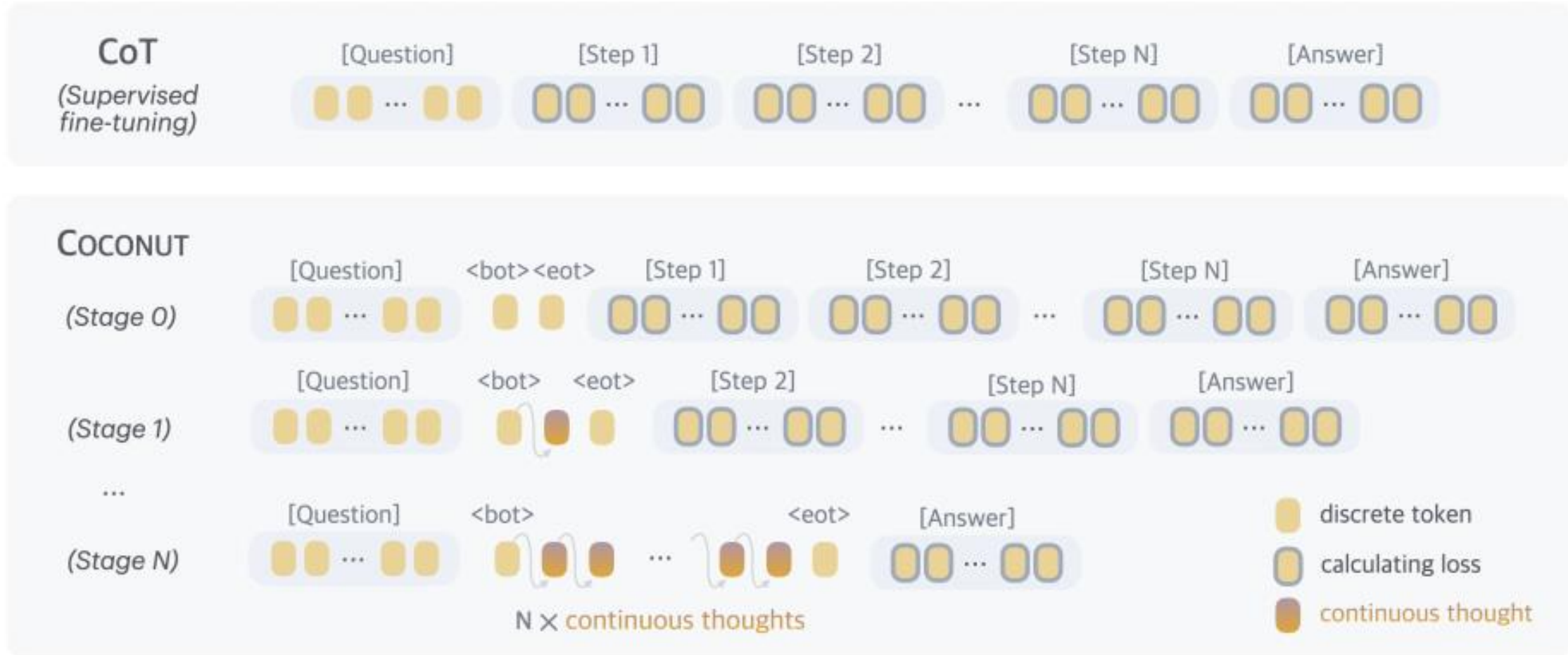
Figure 2 Training procedure of Chain of Continuous Thought (CoCoNUT). Given training data with language reasoning steps, at each training stage we integrate c additional continuous thoughts ( c = 1 in this example), and remove one language reasoning step. The cross-entropy loss is then used on the remaining tokens after continuous thoughts.
